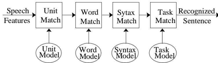
**Figure 3** Block diagram of a typical modular continuous speech recognizer
